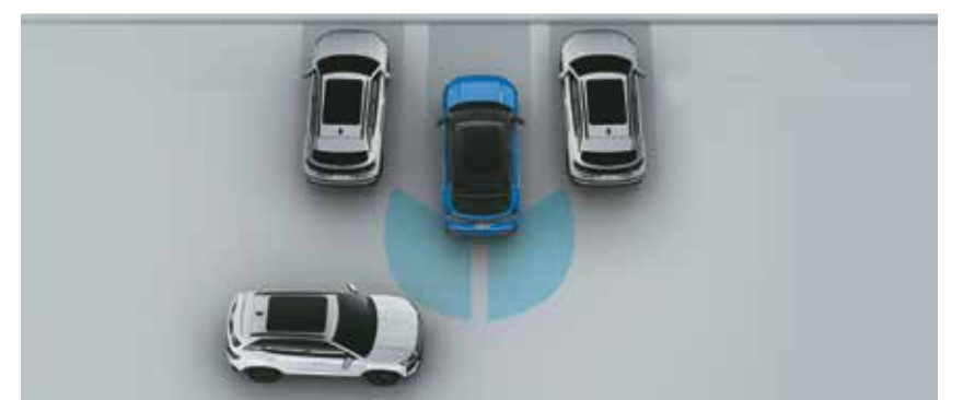
Rear Cross - Traffic Collision - Avoidance Assist (RCCA) & Rear Cross - Traffic Collision Warning (RCCW)
